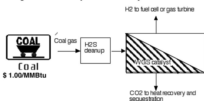
relatively pure for easy sequestration. The design shown is thus a newer version for a FutureGen electric generator, but one with fewer components and that can be scaled to smaller sizes easily.
